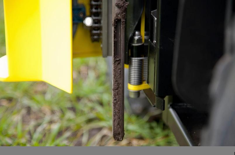
The WINTEX is a hydraulic probe used for fast and precise soil sampling. It samples at a consistent depth, which ensures a complete and homogeneous soil sample.
